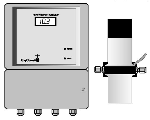
for the measurement of pH in pure water - 1  $\mu$ S/cm
